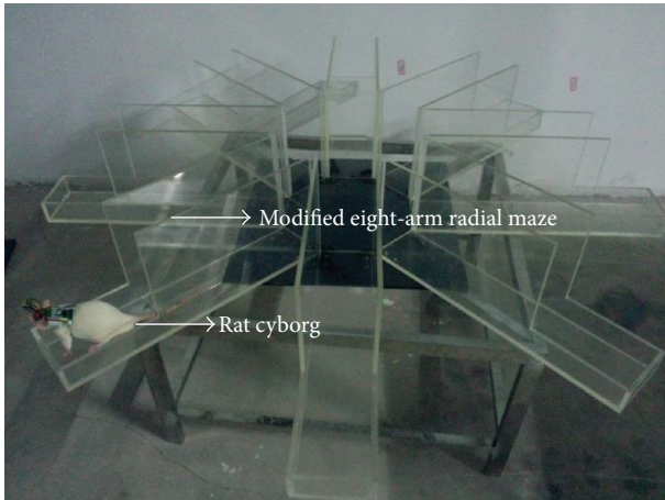
FIGURE 8: A side view of the modified eight-arm radial maze for automatic training. Two high plexiglass walls ( 40\text{ cm} \times 15\text{ cm} ) have been added to each arm ( 60\text{ cm} \times 15\text{ cm} ) to prevent the rat cyborg from climbing up the arm, and the width of each arm is set small enough to prevent the rat cyborg from turning around. Because the plexiglass walls is shorter than each arm, the rat cyborg can turn around at the tail end.
